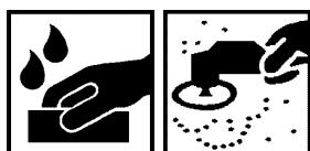
After 3.5-4.0 hours at +20°C, defects and inclusions can be removed with abrasive materials:
